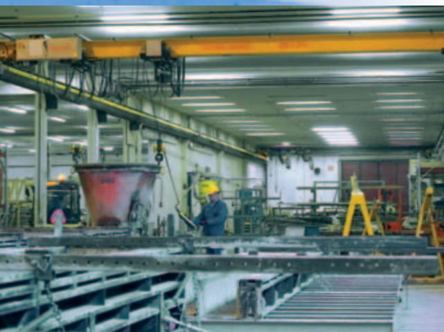
Pre-cast concrete elpo elements are cast in batches for each group of risers. This ensures that pipes, sockets and branches fit properly when assembled on site.
