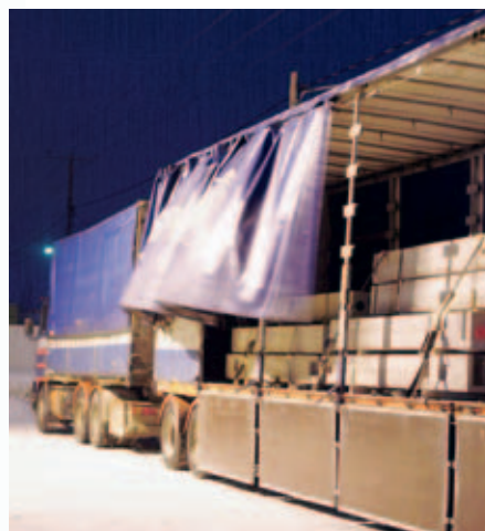
Elpo elements are delivered straight from the factory to the site in storey-height batches.
